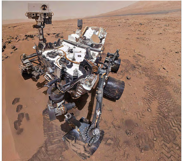
A self-portrait of Curiosity, taken with the MaHLI camera, showing imprints of scooping activities in the sand.
